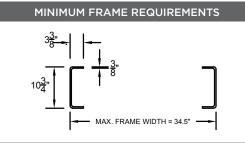
Minimum section modulus per rail =  $17.8 \text{ in.}^3$ Minimum yield strength = 110 KSI
